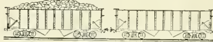
Loaded Car, 150,000 lbs. Empty Car, 40,000 lbs. Braking Power Braking Power 40% on 50 lbs. cyl. pres. 60% on 50 lbs. cyl. pres. Draw Bar Strain 1,837 Lbs.
